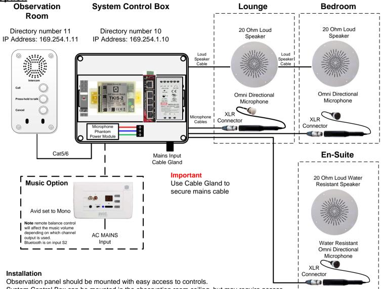
System Control Box can be mounted in the observation room ceiling, but may require access.
