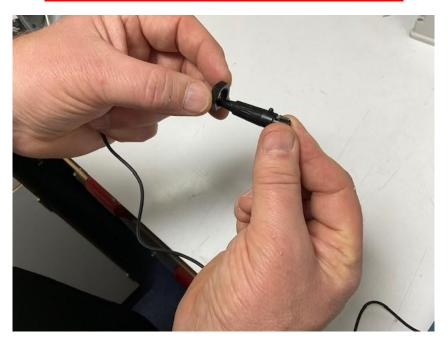
Great Care must be taken when removing microphone locking nut over the mini XLR not to pull on the cable as this will damage very easily and is a common fault when installing.
