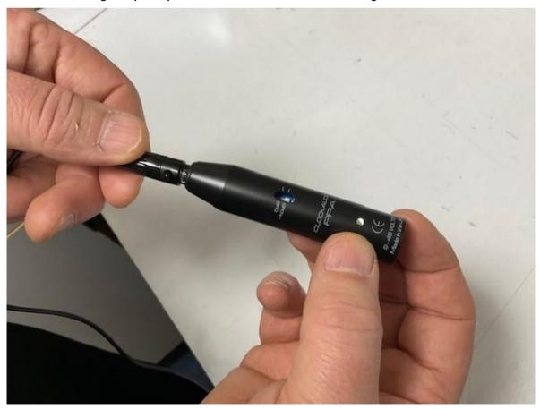
When plugging in the microphone mini XLR to the phantom module be very careful to offer the mini XLR into the socket and turn very gentle until it slides into the socket. The mini XLR does not plug in line with the phantom unit as you would expect. It should not take any effort in insert.
