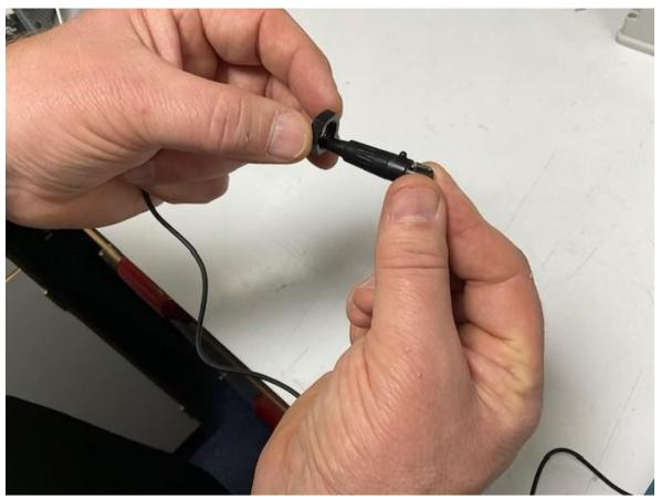
Great Care must be taken when removing the microphone locking nut over the mini XLR not to pull on the cable as this will damage very easily and is a common fault when installing.
