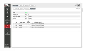
Use the event log or syslog to receive notifications about access attempts or changes in the switch configuration — either by locally tracking them in the event log or by sending messages to a remote syslog server — so you are always up to date on the state of the network.
