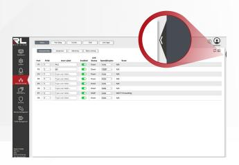
The logical view of the switch can be displayed on any NT5000 web page by simply clicking the <sup symbol located in the upper right corner of the page.
