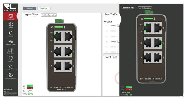
The logical view displays the real status of the system's panel. It can be accessed from the Dashboard and also on any other page by clicking on the left chevron icon at the upper left side of the interface.
