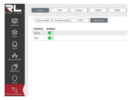
This page allows you to Enable/Disable Telnet and SSH on the switch.
