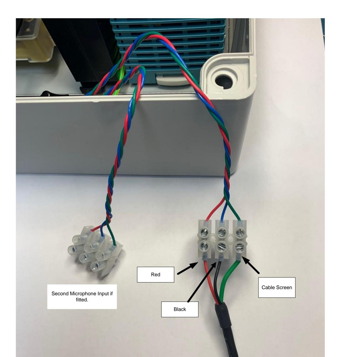
Microphone Connections Parallel Inputs/Mixed Inputs
